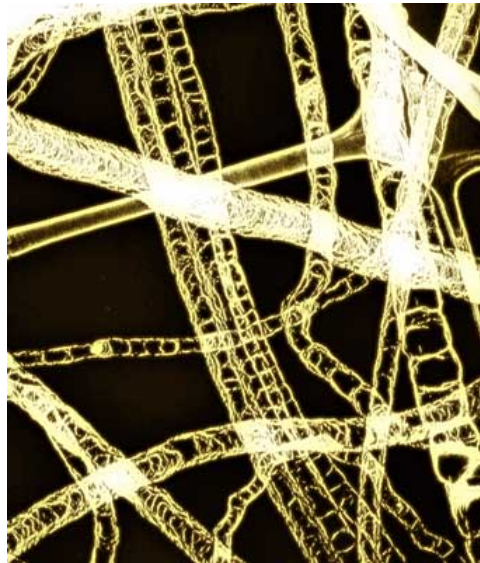
Figure 1. Dark-field image of nitrogen doped multi-walled nanotubes. Copyright Université Paris-Sud, STEM Group.
