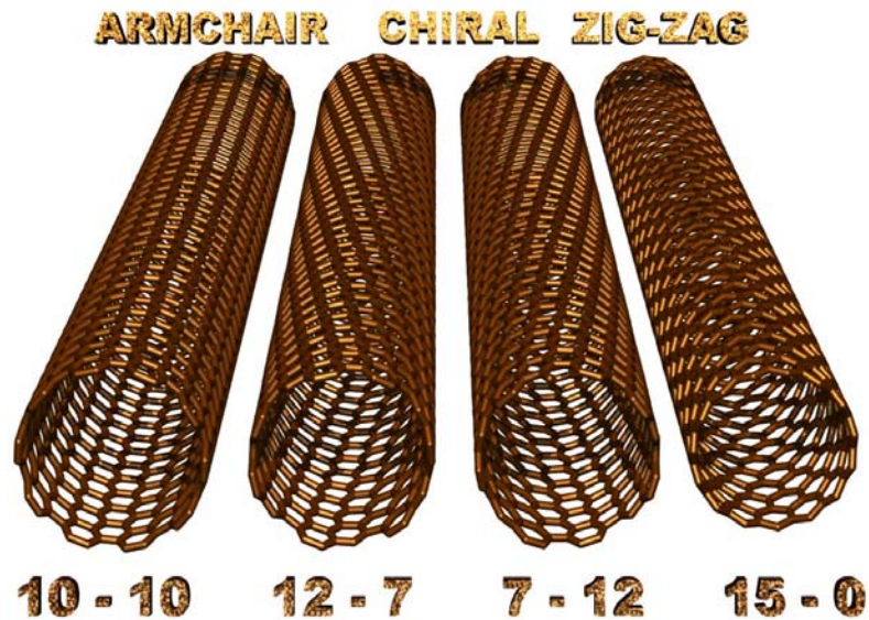
Figure 3. The three types of CNTs are shown [23]. The tube to the left is a so-called armchair ( n = m ), the two tubes in the middle are chiral ( n \neq m ), and the one to the right is a zigzag tube ( m = 0 ). The particular values of the pair of indices ( n, m ) is addressed to each tube. The description ‘armchair’ and ‘zigzag’ come from the circumferential arrangement of carbon atoms.
